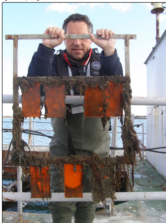
Figure 15: Example of a settlement frame with plates.
