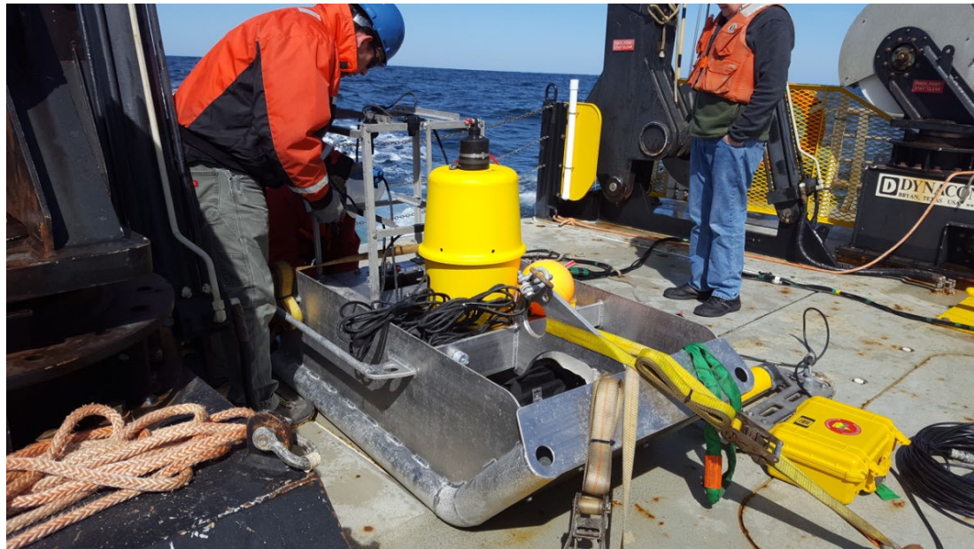
Figure 4: The URI Geosled containing a tetrahedral hydrophone array and 3-axis geophone along with Several Hydrophone Receive Units for data acquisition.
