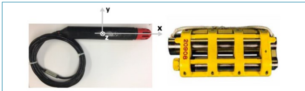
Figure 25. Close up view of the three-axis geophone (right panel) and OBX system (left panel)
