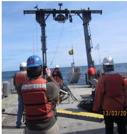
Figure 5. Geosled to be deployed 1 km from A01 and A02 turbine locations to measure acoustic and seismic signals from impact pile driving
