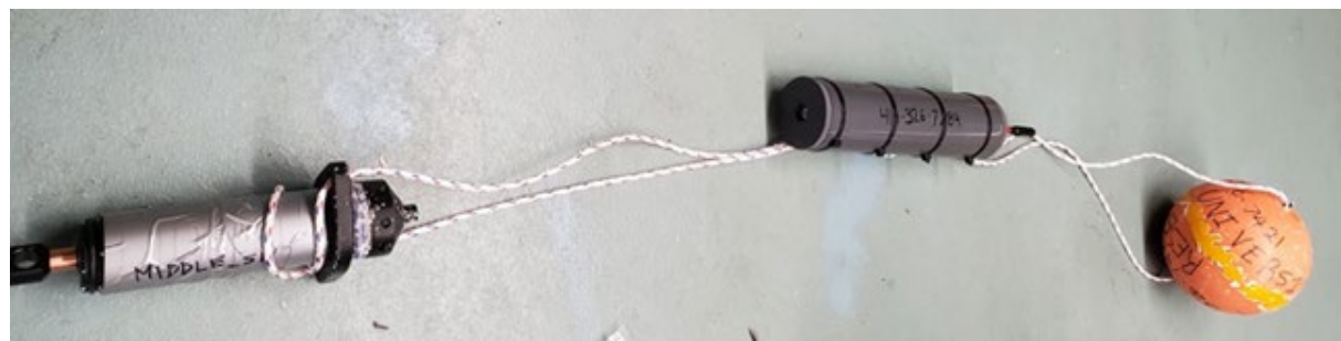
Figure 8. Photograph of the mooring with the acoustic release at the bottom (left side of image), the LS1 acoustic recorder in the center of the line, and a sub-surface buoy at the top (right side of image).
